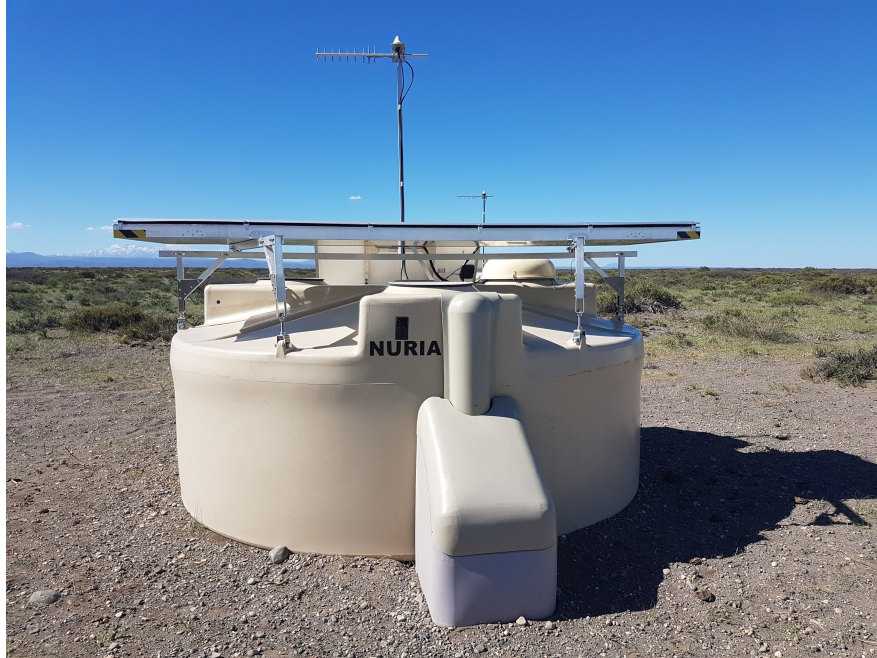
Figure 3.3: A water Cherenkov station fitted with a scintillator detector as part of the AugerPrime upgrade [22].
