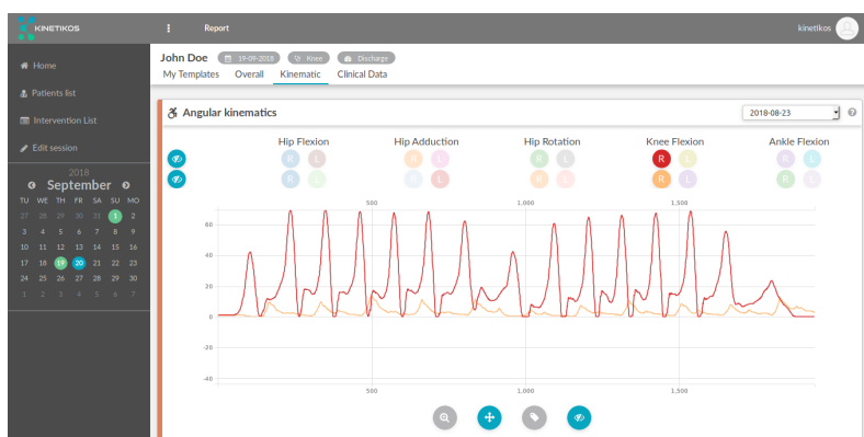
Figure 5.7: Example of an hypothetical Kinematic report tab, with knee flexion highlighted for both the admission (orange) and discharged (red) sessions.
