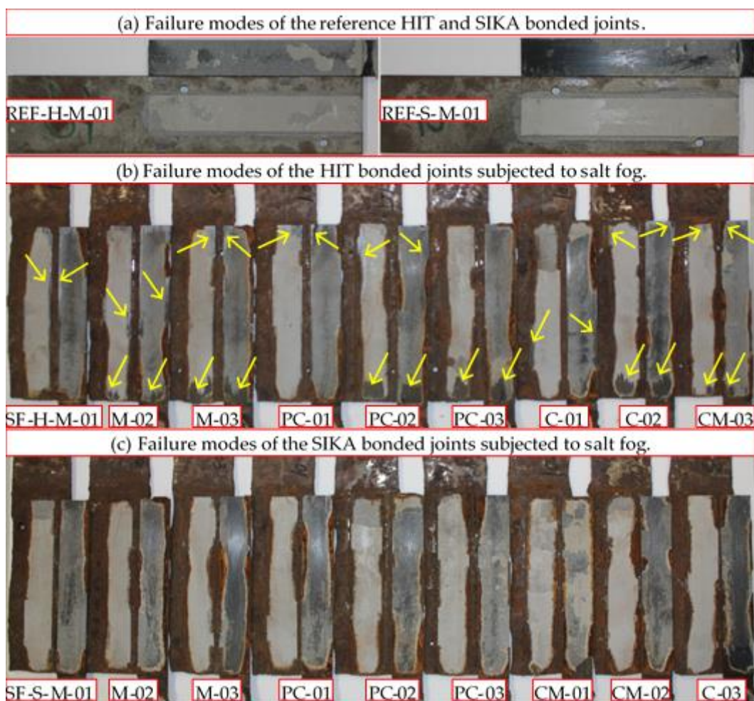
Figure 5.3 - Failure modes of (a) the reference and aged bonded joints with (b) HIT and (c) SIKA.
