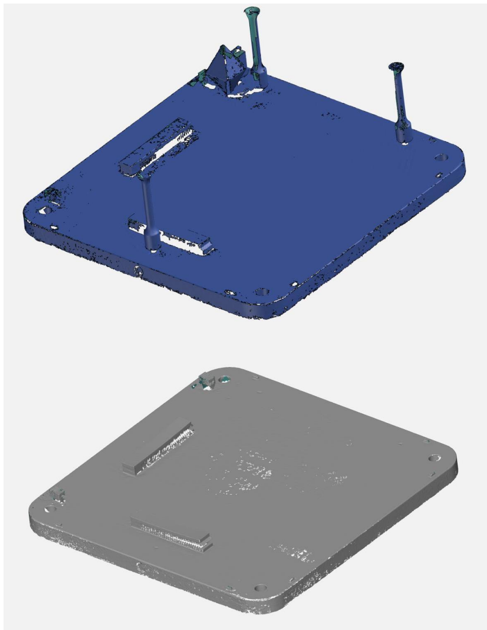
Figure 4.2 Calibration samples before and after cutting (a) top half; and (b) bottom half.
