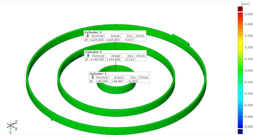
Figure 4.16 Simulation optimization result (-0.5 mm to 0.5 mm scale)
