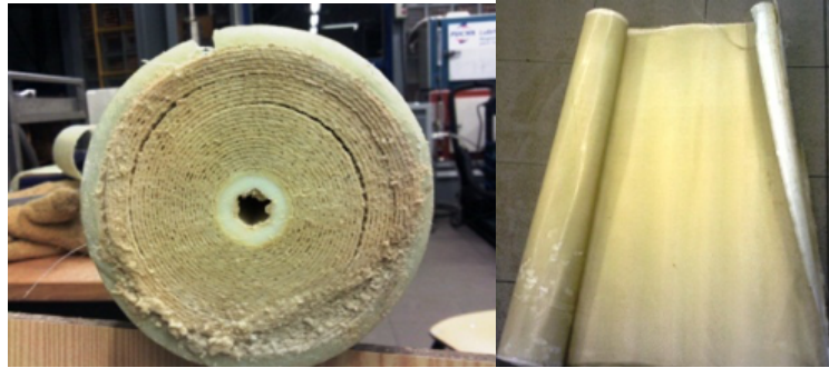
Figure 5-8. Images of the module membrane sacrificed for autopsy and characterisation of fouling.
