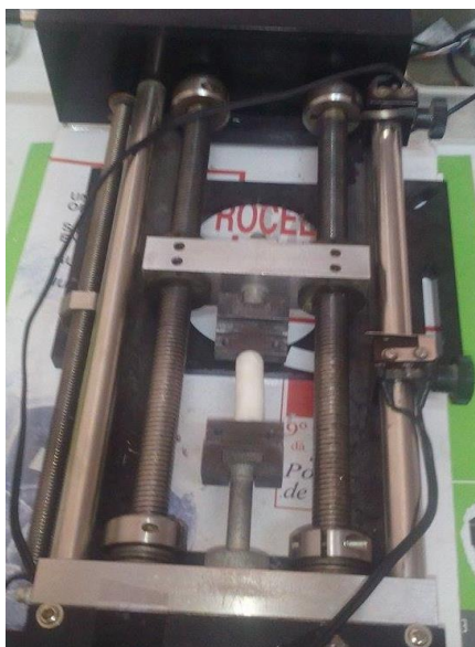
Figure 2.7- Mechanical tester and scaffold
