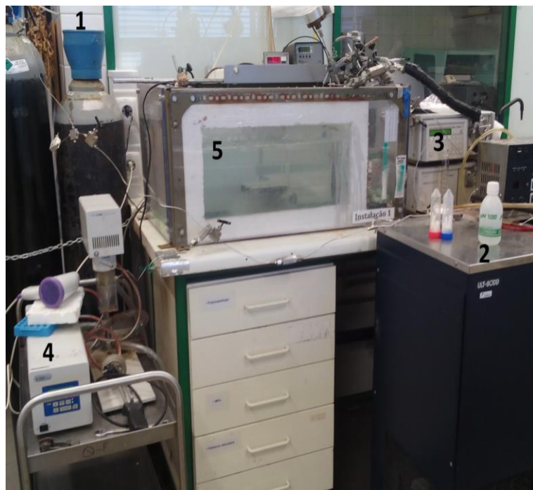
Figure 2.4--ScCO 2 apparatus; (1) CO 2 bottle, (2) cryostat, (3) pump, (4) back pressure valve, (5) thermostated bath
