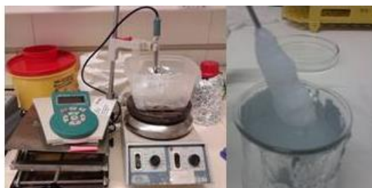
Figure 4.3. (Left) Assembly of the experiment and (right) pellet recovered after methacrylation.
