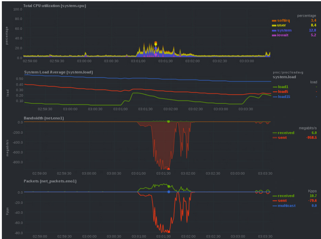
Figure 5.6: System metrics for one run on the iCBD-Cache02 in a boot storm scenario
