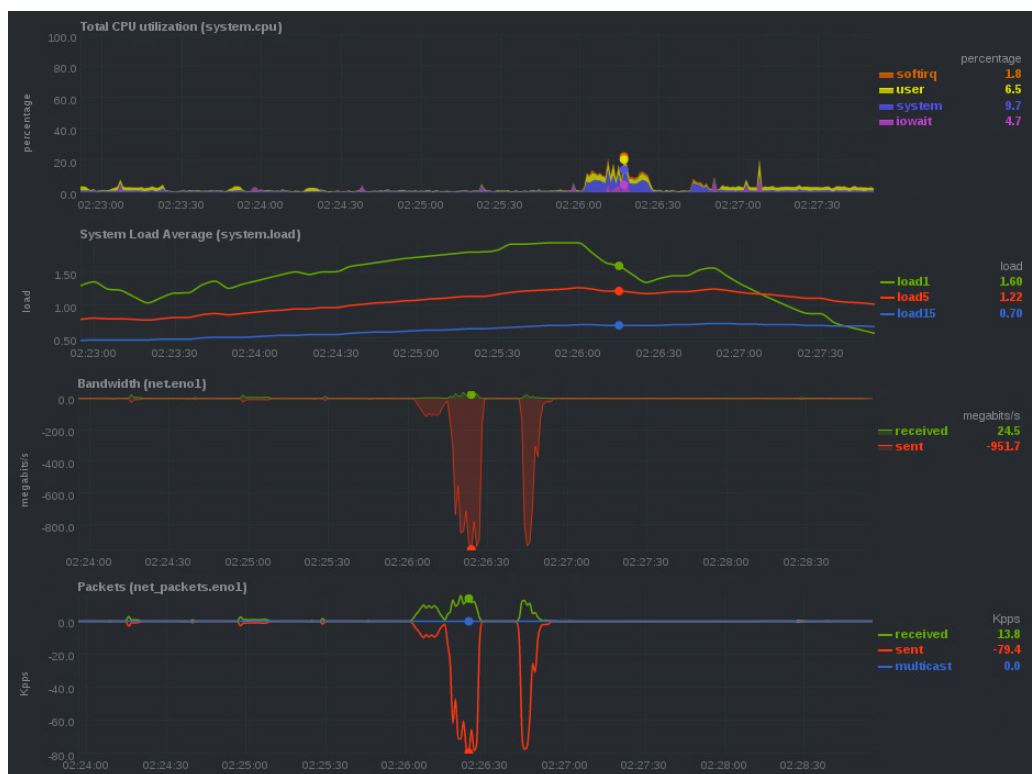
Figure 5.5: System metrics for iCBD-Cache02 on one run of the five workstations sequential boot scenario test
