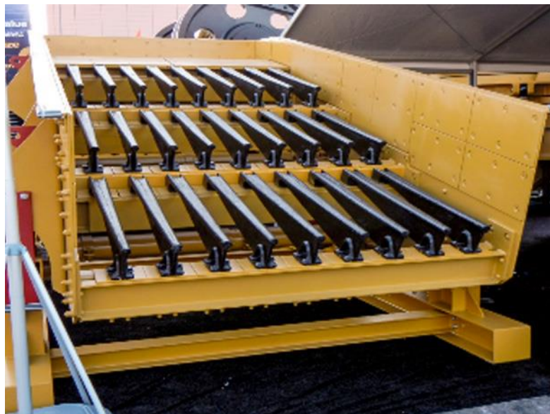
Figure 13 Grizzly bars 3 stages screen (Taken from ( https://www.dismet.com/productos/precibadores/ )).
