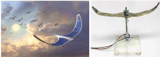
Figure 6. An artist's rendering of the solid-state aircraft (left) and two little wings, each 5 centimetres long, fabricated out of ionic polymer-metal composite (right)
