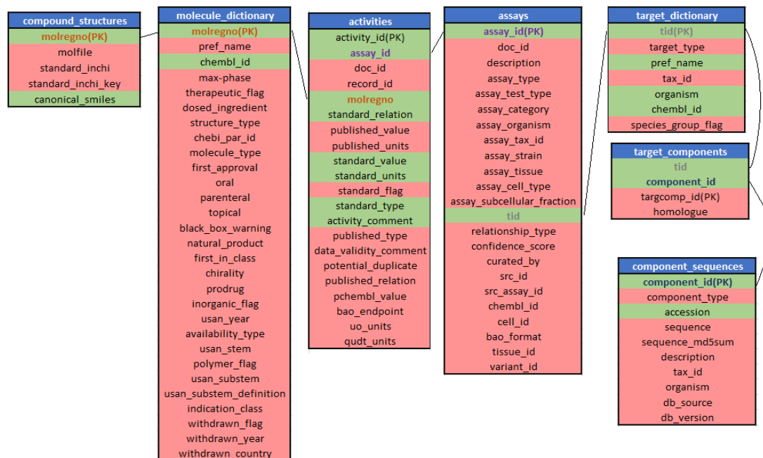
Figure 5.1: Seven retrieved tables from ChEMBL_23. Green background represents selected columns and red background represents unselected. The lines between columns represent the columns that inter ligate all table information.
