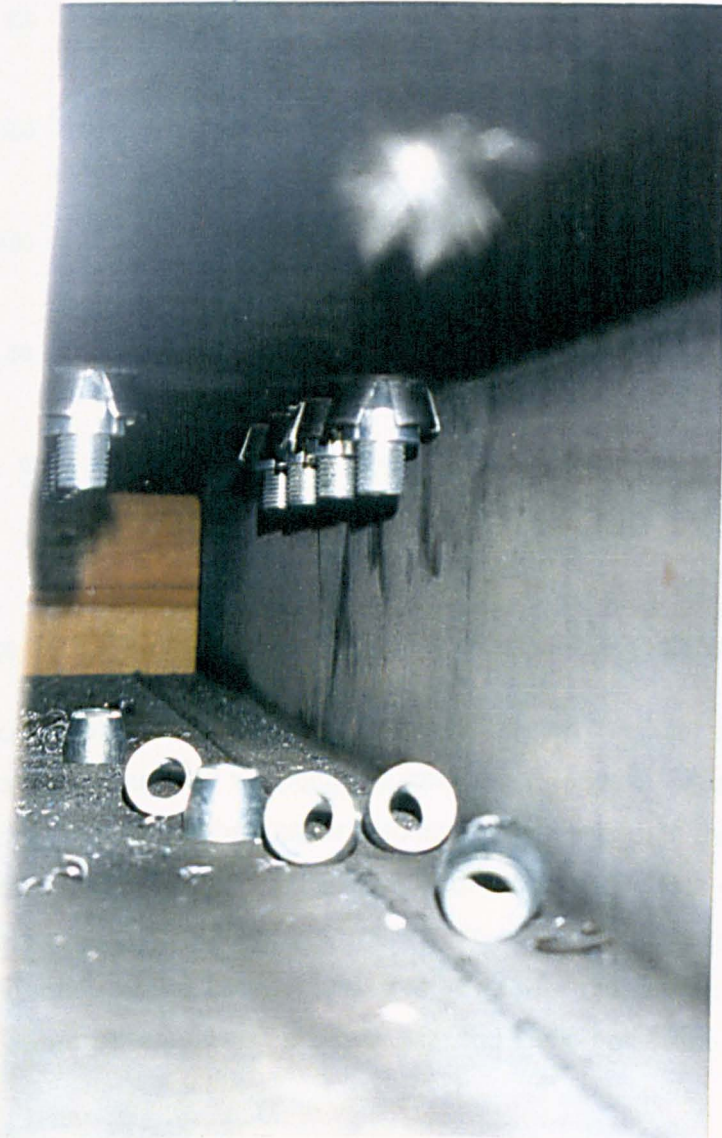
Figure 5.20 Premature Hollo-bolt pull out photographed from inside the column
