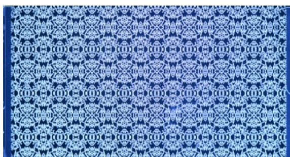
Figure 4.4. Image of an empty micromodel taken with the DSLR camera set-up.
