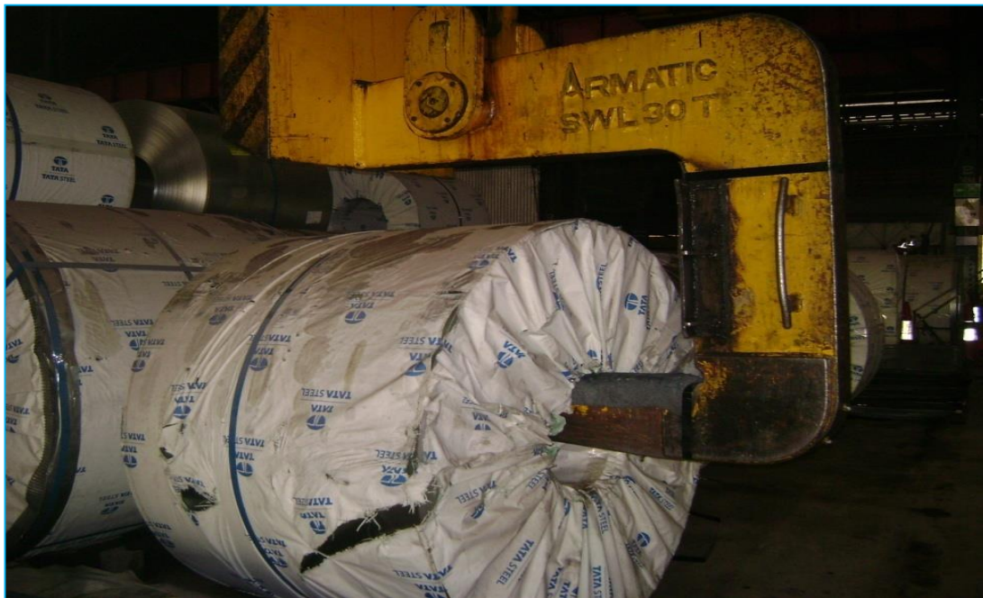
Fig. 5.1. Inserting “C” hook into coil bore
