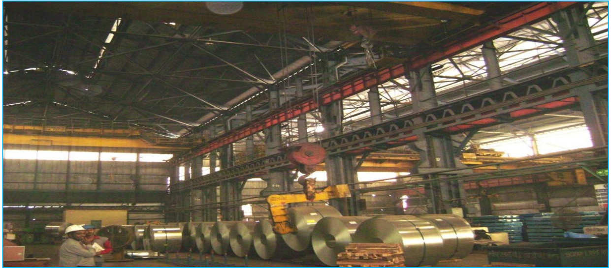
Fig 1.1. MATERIAL HANDLING WITH EOT CRANE USING “C” HOOK
