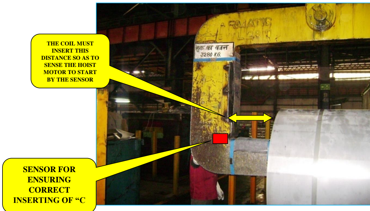
Fig 5.3. Suggest Figure of handling coil with complete inserting of “C” hook
