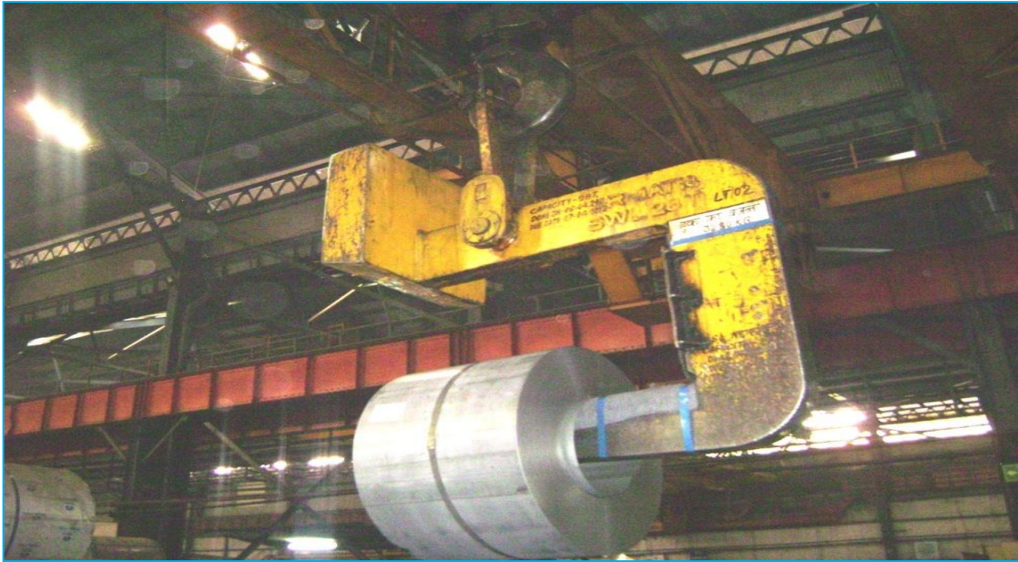
Fig 5.2. Handling coil with incomplete inserting of “C” hook arm
