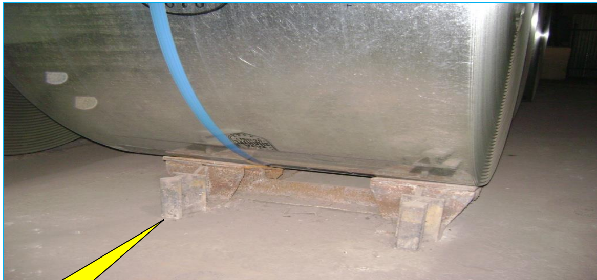
Fig 5.5. Off center coil placement on saddle
