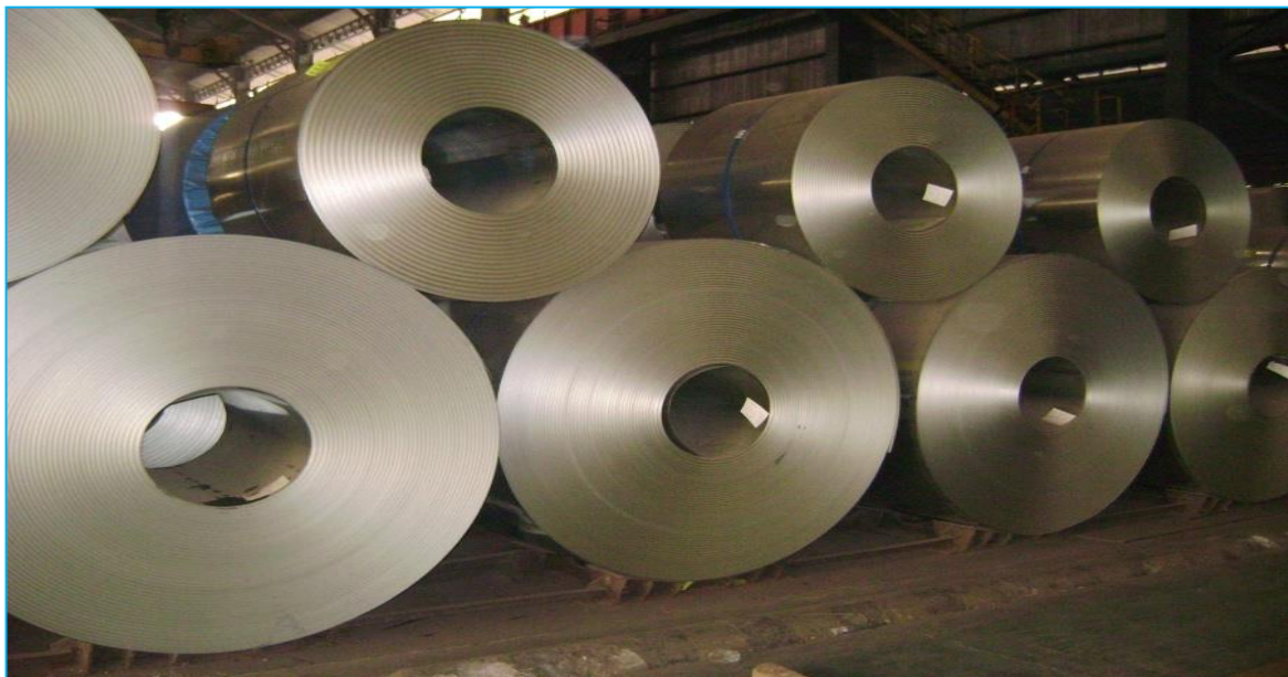
Fig 5.4. Storage pattern of coil on the saddle
