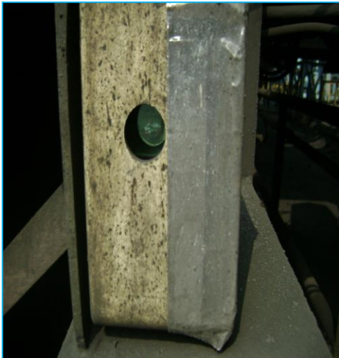
Fig 5.9.Laser Sensor Of Anti Collision Equipment
