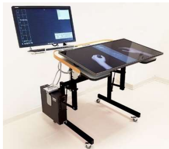
Figure 3: The Promotœr comprises a computer, a screen for the therapist feedback (EEG and EMG activity monitoring) and a screen for the ecological feedback to the patient (a virtual hand performing the imagined movement in successful trials). A commercial wireless EEG/EMG system (gTec, Austria) is used to record brain and muscular activity from the patient.
