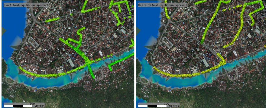
Fig. 3. Result of penalizing risk in the simulation: Agents use the dangerous bridge in the left case, but avoid it if its usage is more costly. In the right case, crossing the bridge is costly ( r_j > r_i in eq. (8), i.e. node j will be flooded earlier than node i ).
