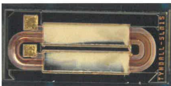
Figure 7. a micro-magnetic inductor integrated on silicon. The inductor consists of a racetrack shaped copper coil, which is surrounded by a layer of magnetic material.
