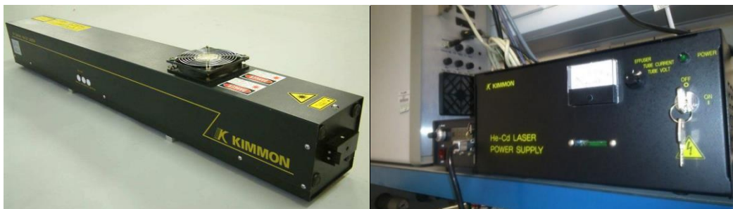
Figure 2-23 IK Series He-Cd Laser and power supply used in this thesis.
