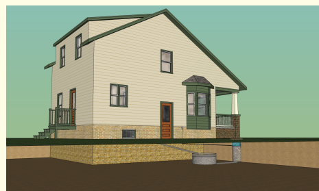
Figure 3. MFC system installed in a three people household. It consists of two elements both under the ground. The two elements are a buffer tank that will store the water and using a valve will pump it, with a regular flow rate, to the hybrid-up-flow MFC. This way it will avoid the fluctuations of the wastewater generation during the day. No agitation will be needed because the height difference will contribute to the homogenization of its content every time the wastewater arrives to the tank. There will be a closed water circuit and electricity net [Sketch created by Google SketchUp version 8].
