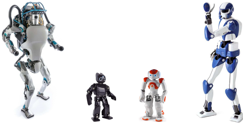
Figure 1.1 Examples of state of the art humanoid robots. From left to right: Boston Dynamic Atlas, Robotis Darwin-OP, SoftBank Robotics Nao, Kawada Industries HRP-4
