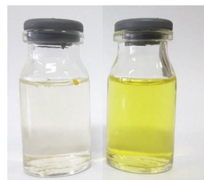
(b) Image of the aqueous dispersions containing curcumin (right) and the curcumin solid dispersion (left).
