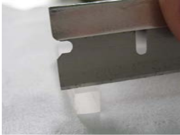
Figure 3.7: A bar of \text{BaF}_2 before cleaving it with razor blade.
