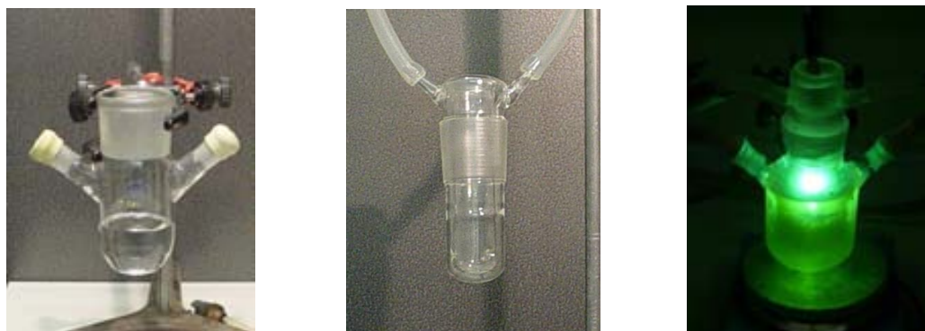
Figure ES2. Photochemical reactor, refrigeration jacket and photochemical reaction.
