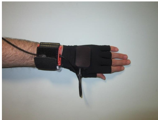
Figure 5.17. Xsens MVN Biomech Suit. Positioning of the inertial sensors above the metacarpals and at the distal end of the radioulnar segment to define the wrist joint.
