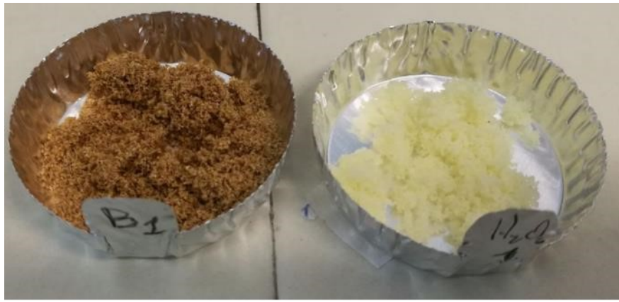
Figure 13. Blank reaction on the left (sodium hydroxide). Rice husk treated by alkaline hydrogen peroxide on the right (sodium hydroxide/hydrogen peroxide)
