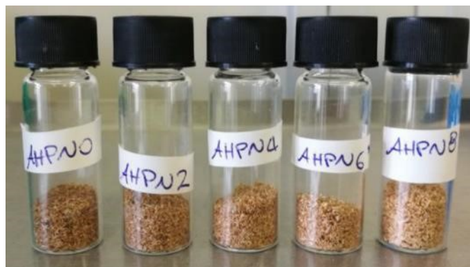
Figure 11. Rice husk samples treated with the ammonium hydroxide (15%) and hydrogen peroxide mixture. From left to the right hydrogen peroxide concentration increases. Slight colour change is noticeable.
