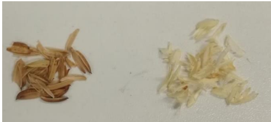
Figure 14. Raw whole rice husk on the left. Whole rice husk treated by alkaline hydrogen peroxide on the right (sodium hydroxide/hydrogen peroxide)
