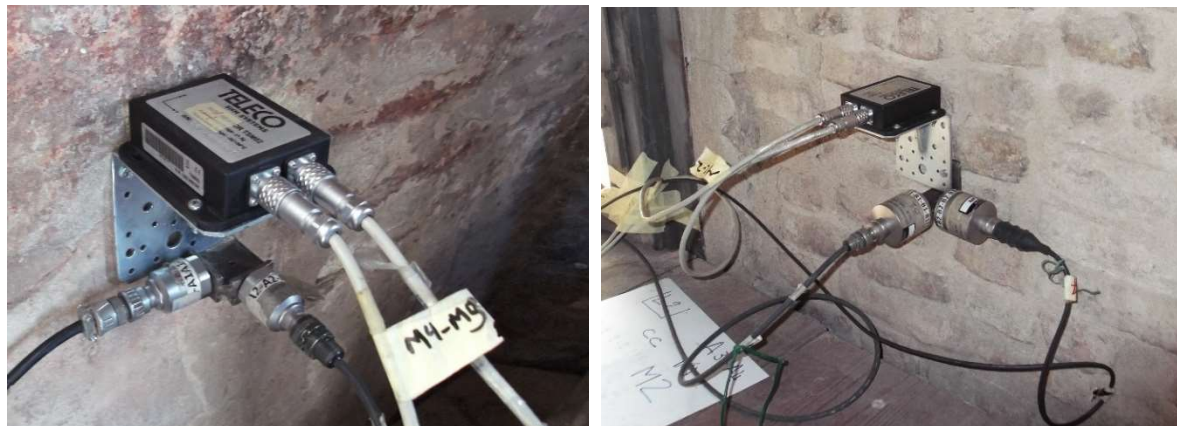
Figure 7. Typical installation of MEMS and piezoelectric sensors.
