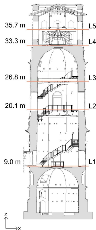
Figure 5. The instrumented levels (L1–L5).
