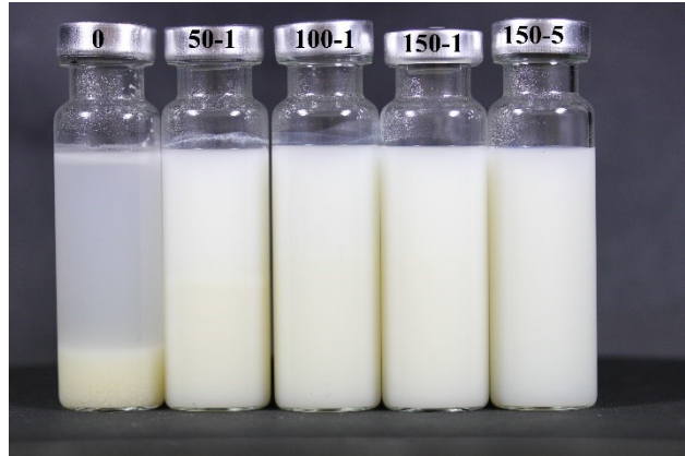
Figure 9. Phase separation of 10% (w/w) untreated okara aqueous dispersion and samples submitted to HPH treatments at 50, 100, 150 MPa pressures and 150 MPa with 5 passes during 1 day storage at 4 °C.
