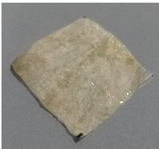
Figure 24. Visual appearance of supercritical-CO 2 -dried lettuce waste after immersion in water.
