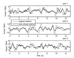
Experimental tests lead to the conclusion that the developed look-ahead method can limit the acceleration values at the joints, and allows to reduce the values of the motor torques at the robot joints. The reduction of the RMS value of the motor torque can reach values as high as 30% when compared to the original manufacturer's proprietary method.
