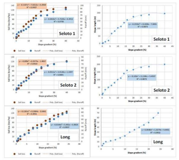
Very steep slopes (> 20% to < 40% gradient; > 50 m slope length): are prone to mass movement, severe rain splash and sheet erosion.
