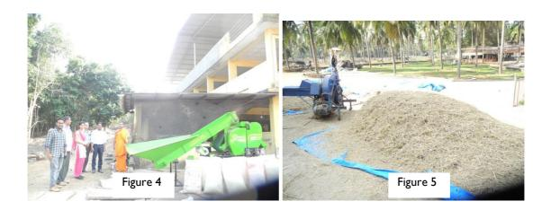
The sundried grass (moisture 40%) brought by the Municipality (at their own cost) was chopped using a 10 HP chaff cutter (Figure 5) and mixed with locally available legume haulms (ground nut/ mung bean /green gram) in the ratio 65:35. The chopped mixture was then fed to the mini baler cum wrapper, which compressed and wrapped the grass legume mixture to 40 kg bales (Figure 6, 7).
