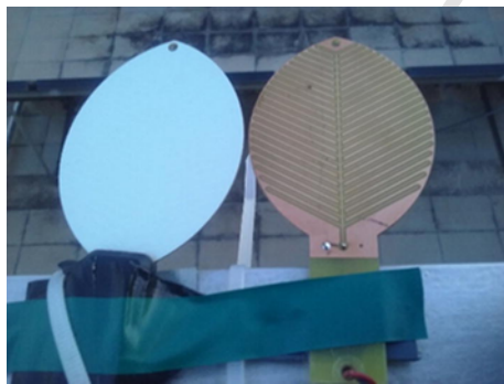
Fig. 9. Model B (left) and OVAL (right) sensors ready for the wetting-drying experiment.
