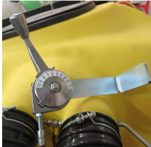
Fig. 15 – Example of device for adjusting the dust rate (Photo: DiSAFA)
