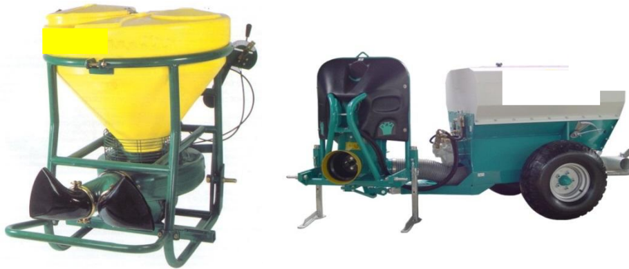
Fig. 1 - Example of conventional duster (category A) (Photo: DiSAFA)
