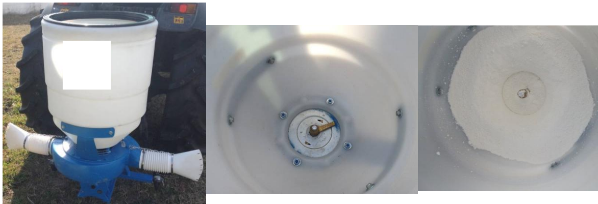
Fig. 11 – Example of mechanical agitation system (Photo DiSAFA)
