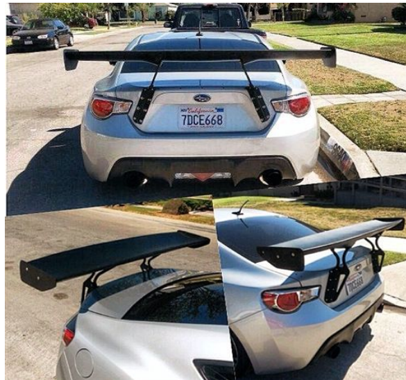
Figure 5.6.2: Example of a rear wing
