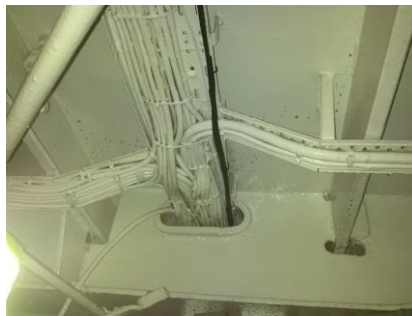
Figure 4. Electrical distribution layout in a 1047 GT tug vessel
