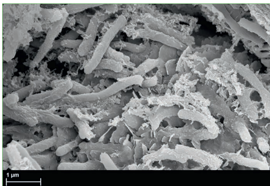
Figure 2 Scanning electron micrograph of microorganisms on corroded carbon steel (AISI 1030).
