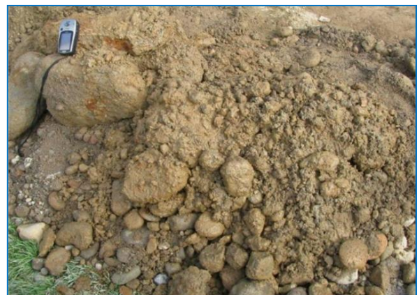
Fig. 6 Cobbles and boulders collected during the excavation
