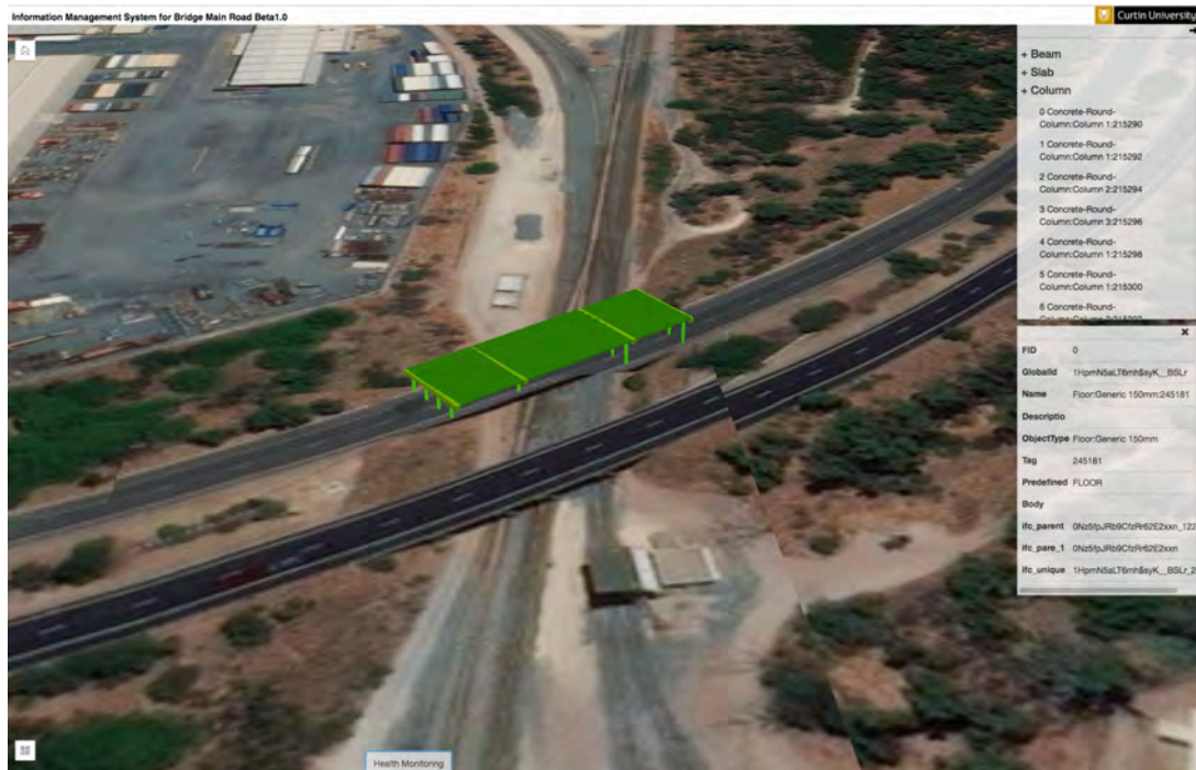
Figure 7-15 Bridge 1 management system for Main Roads WA.
