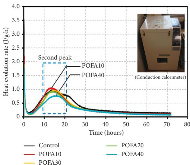
FIGURE 5: Heat evolution rate of mortars containing mPOFA.
