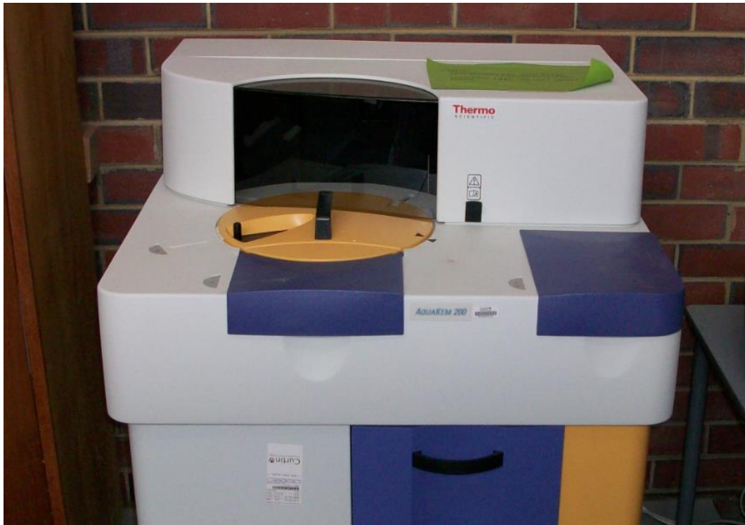
Fig.3.4.: AquaKem machine for testing Ammonia, Nitrate & Nitrite
