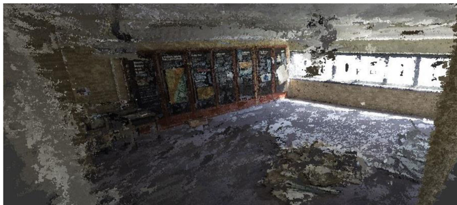
Fig. 3 An example of reconstructing 3D point cloud (A point cloud is a set of data points in some coordinate system. In a three-dimensional coordinate system, these points are usually defined by X, Y, and Z coordinates, and often are intended to represent the external surface of an object. Point clouds may be created by 3D scanners (Wikipedia))
