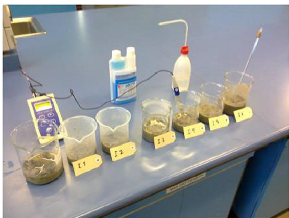
Fig. 2. Initial Cement Consumption (ICC) tests.
