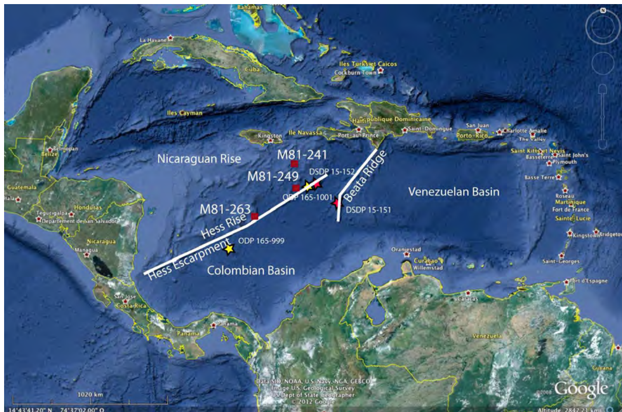
Figure 32: Localization map of the Hess Escarpment and Beata Ridge (yellow stars correspond to ODP sites and red stars to DSDP sites). The red squares correspond to the dredging locations where strontium isotope ratios could be obtained. (Map from Google Earth).
