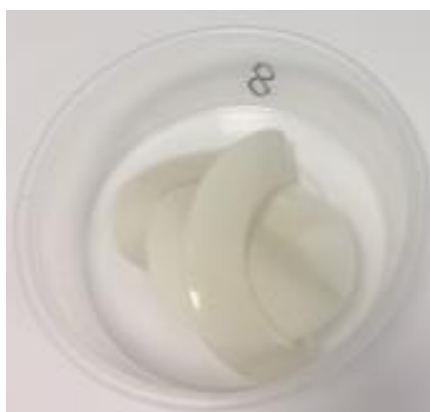
Figure 5.11: Polymer C for QXRD became a thin film of plastic after dried
