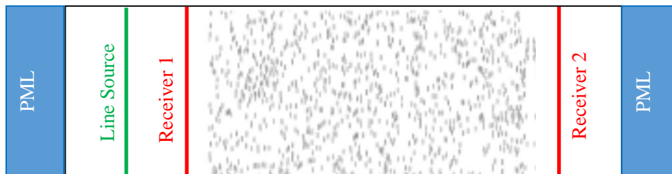
Figure 6-2. Sample configuration for numerical wave propagation simulation (Caspari et al., 2017).
