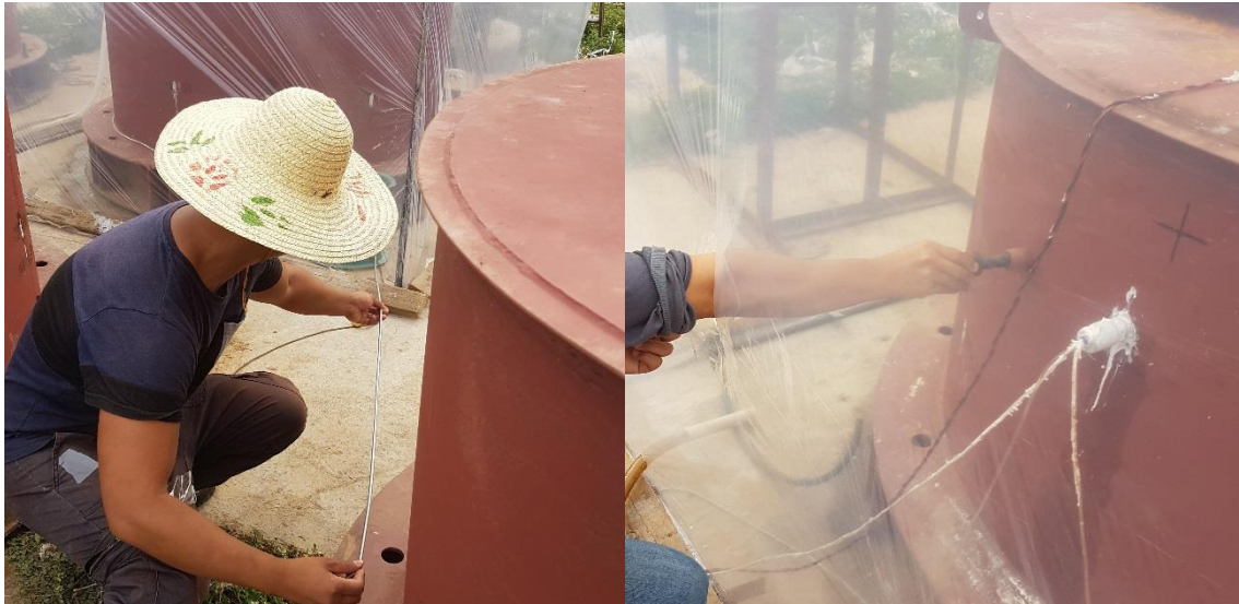
163 (a) Measurement for the confined region (b) Measurement for the tank after mixing 164 165 Fig. 10 Methane-air mixture concentration measuring procedure
