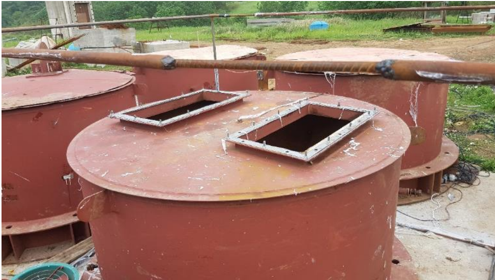
(a) Venting areas on the tank top
