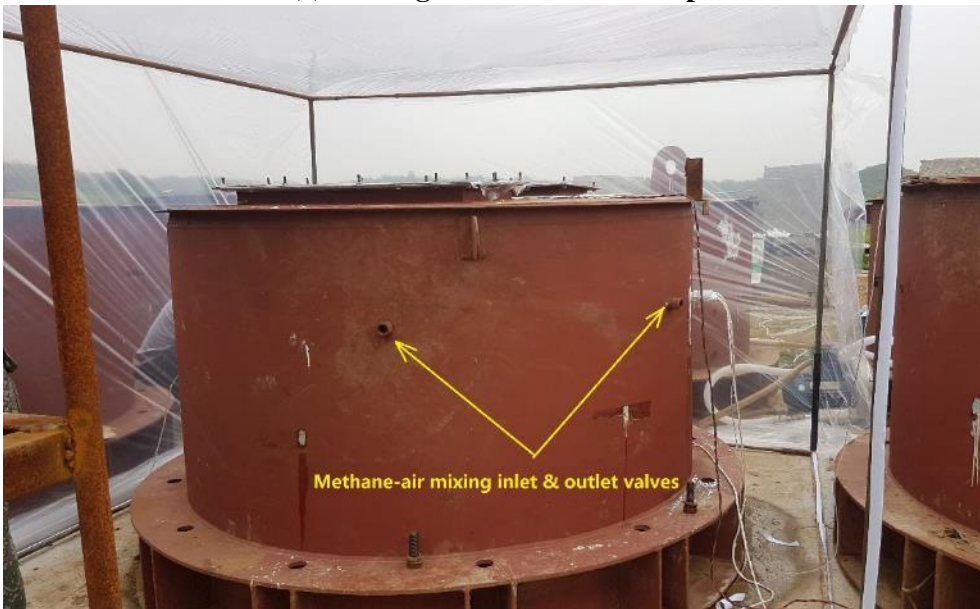
(b) Methane-air mixing inlet & outlet valves
