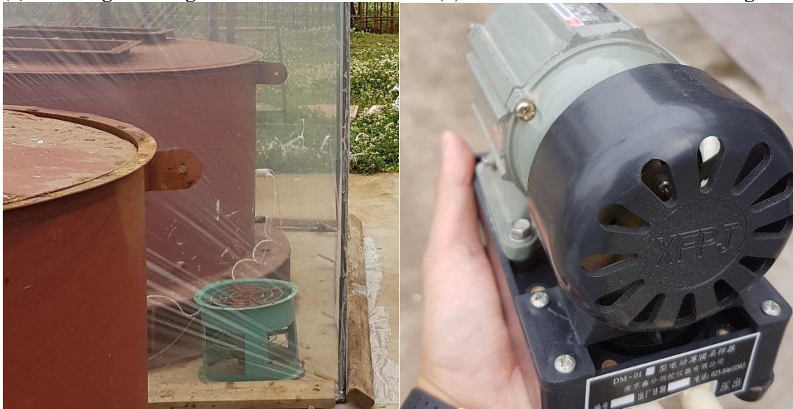
(c) Fan for gas mixing for the confined film region
