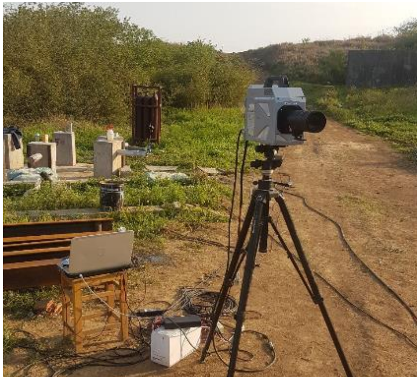
Fig. 7 Location of high speed camera, computer system and compressed gas resources
