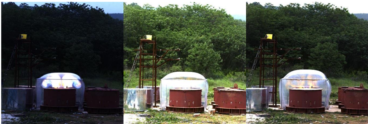
241 242 (a) 500mm separation gap (b) 750mm separation gap (c) 1000mm separation gap 243 Fig. 14 High speed video camera snapshots of different separation gap scenarios in gas explosion 244 testing
