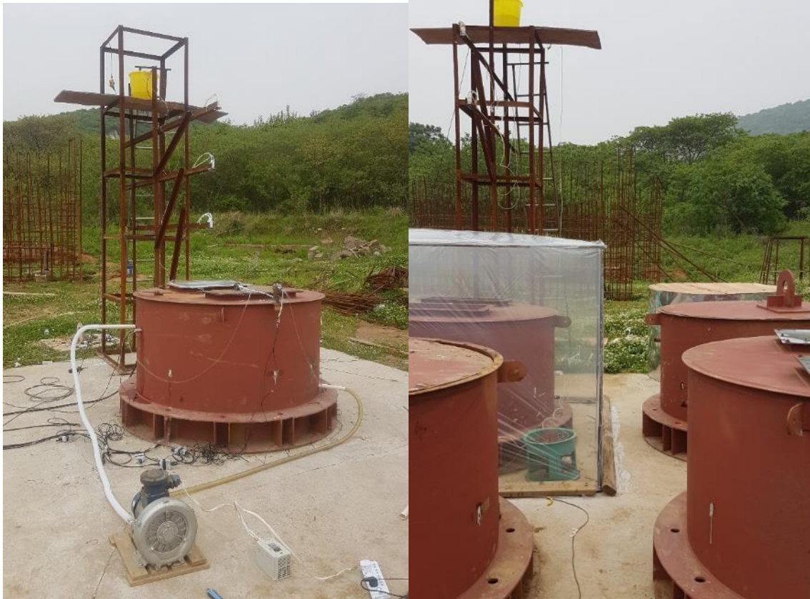
Fig. 5 Locations of fans for gas-air mixing
