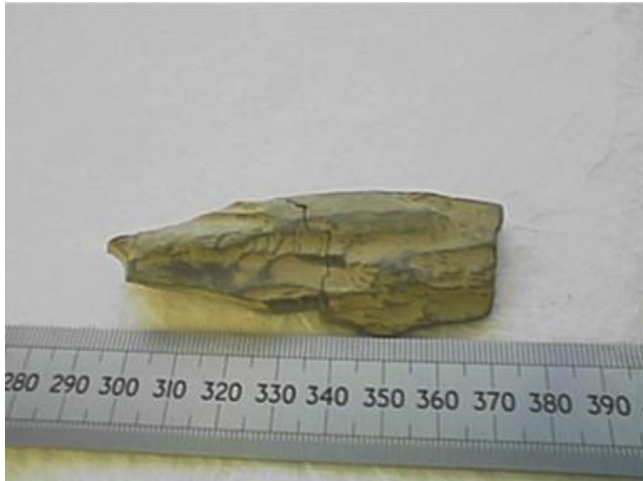
Fig. 3. Angular caving (Bradford et al., 2000).
