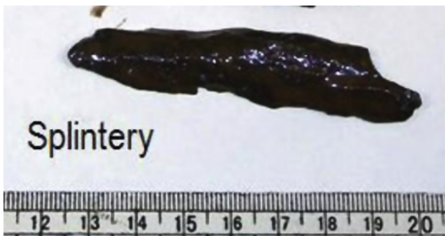
Fig. 4. Splintery caving from underbalanced drilling (Kumar et al., 2012).
