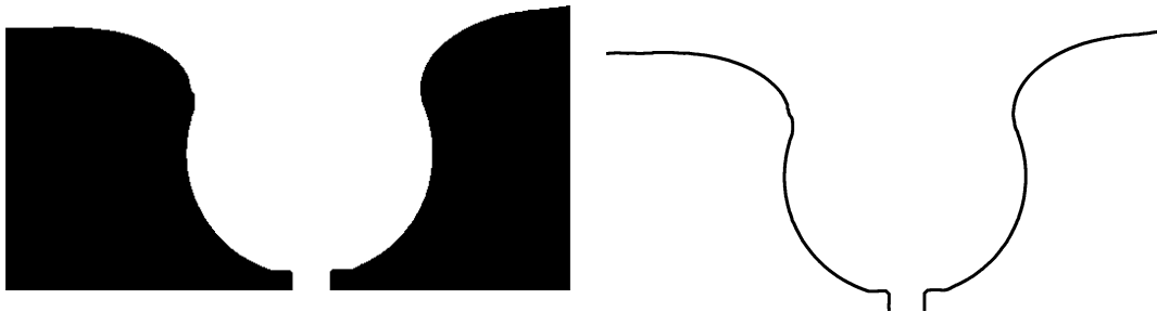
Figure 7.8: (a) the “WIM” mask and (b) corresponding perimeter mask. The perimeter was enlarged using a disk-shaped structuring element with a radius of 5 pixels.
