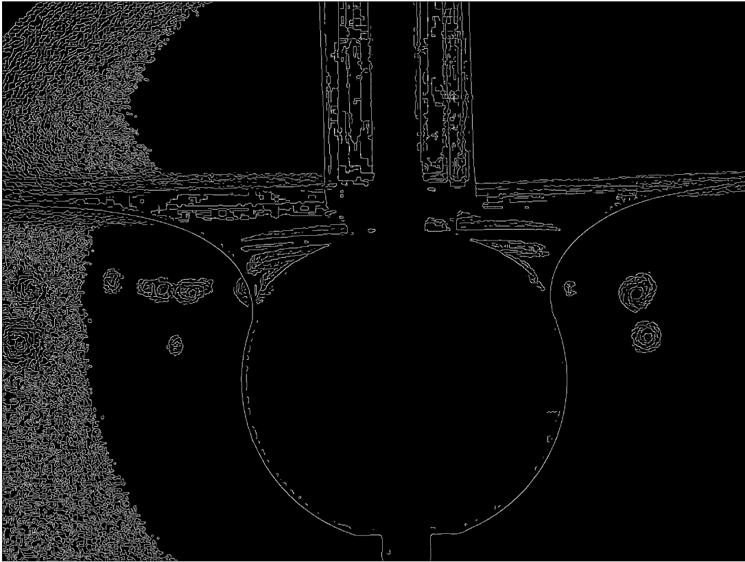
Figure 7.3: Results of Canny edge detection of the image in FIGURE 7.2 using the default thresholds. 3906 individual edge sections are shown in this image, the largest consisting of 1394 pixels and the smallest of only a single pixel.
