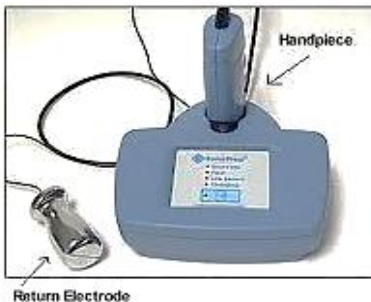
Figure 1.12 SonoPrep skin permeation device: rapid local anaesthesia by ultrasound enhanced delivery of lidocaine (Sontra Medical Corp, Franklin, MA)
