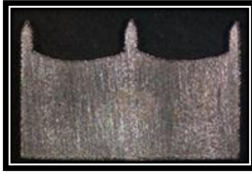
Figure 3.3 MN plate with three 700 \mu\text{m} length \times 250 \mu\text{m} width MN.
