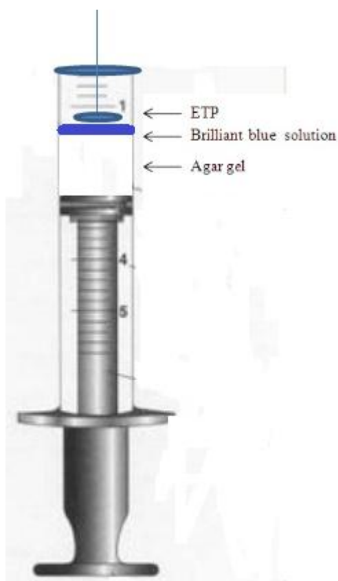
Figure 4.5 Study setup for Agar gel pilot studies
