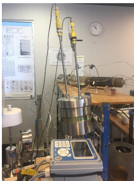
Figure 3-17 Photograph of Rosemount 56 pH meter with two sensors and high-pressure reactor.
