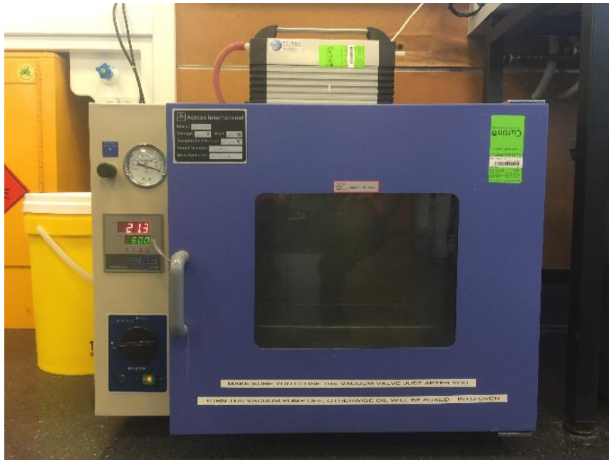
Figure 3-11 Photograph of the vacuum drying system that included an oven (Model VO-16020) and a vacuum pump (Model TW-1A), both made by Across International.
