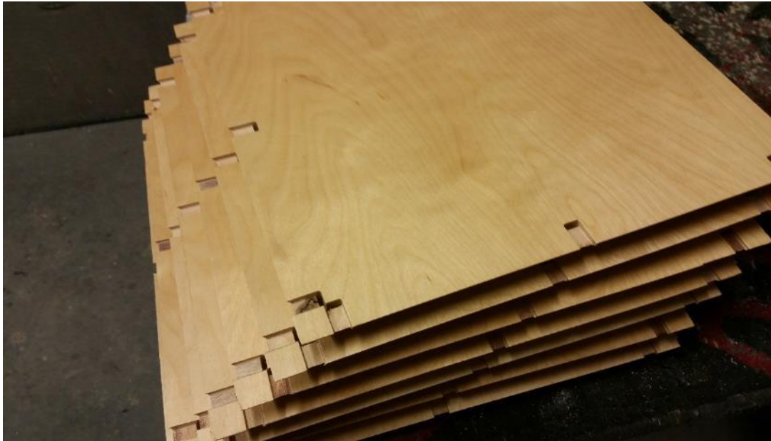
Figure J-7. Forlano, Penelope. Panels routed and sealed, 2017.
